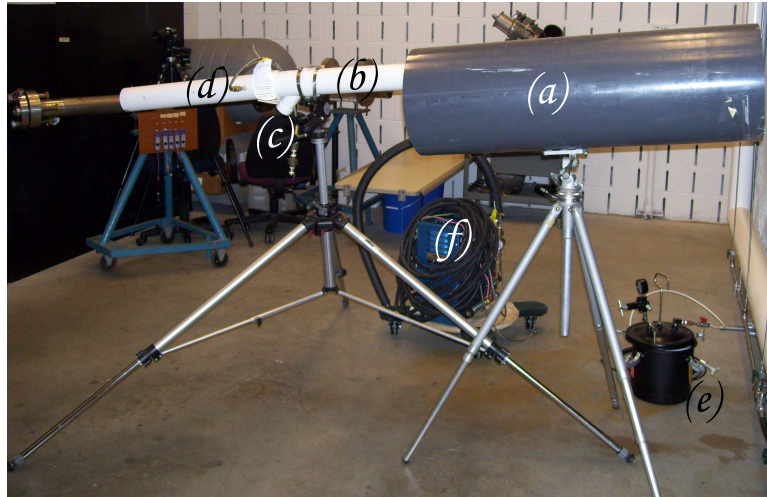
Figure 11. Second seeder configuration that used a large outer cowl to stabilize the flow.
